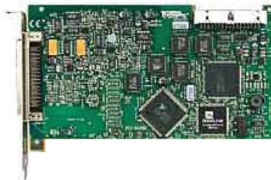
Рис. 3. National Instruments 12-digit A/D converter NI 6023E
